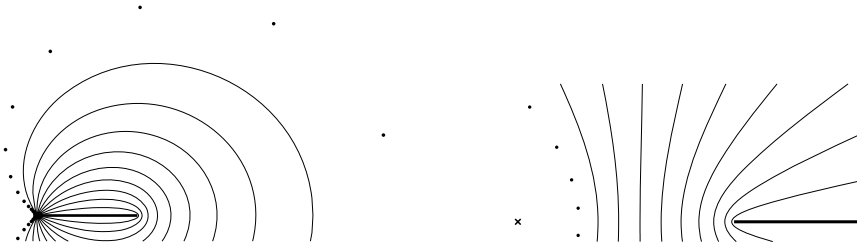
FIG. 9. On the left, repetition of the right panel of Figure 4, now with curves shown inside the quadrature points. If the eigenvalues of \mathbf{A} are not confined to the real interval [m, M] (solid line) but lie within the innermost curve, for example, then Method 2 will still converge exponentially with a rate 90% as fast as before. The next curve corresponds to 80%, then 70%, and so on down to 10%. On the right, a closeup of the same figure near the origin (marked by a cross).
